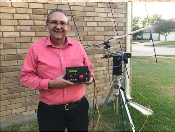
It was truly an exciting moment for me. It was very easy to do. I was using an arrow antenna mounted on the antenna tracker platform I demonstrated at last year's "Show and Tell". It just points the antenna in the right direction and gives me an extra hand to write with. The radio was a Kenwood TH-D74A handheld with 5W output. I hope you and others have the joy of making an ISS contact soon.
